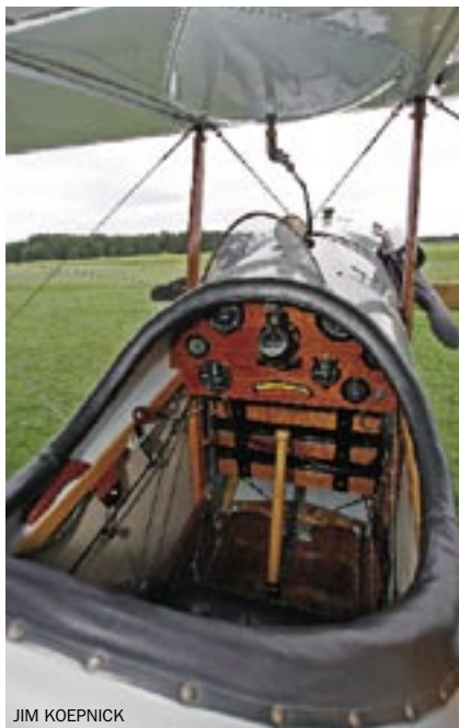
A standard Jenny "dashboard". This is the forward cockpit. All the instruments are original to Navy aircraft of the period.
